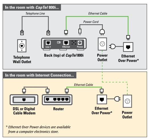
**IMPORTANT:** The Ethernet Over Power devices cannot be plugged into a power strip, surge protector, extension cord or GFI-type outlet. They must be connected directly into the electrical wall outlet.
